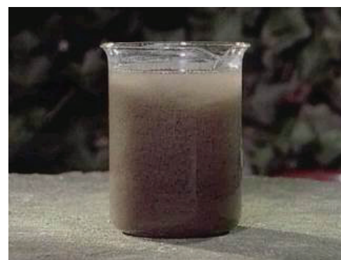
Fig. #2 - Suspension of Activated Sludge
