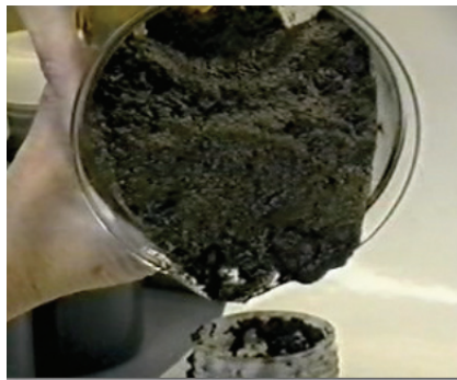
Fig. #6 - Polymer Thickened Sludge (~5% TSS)
