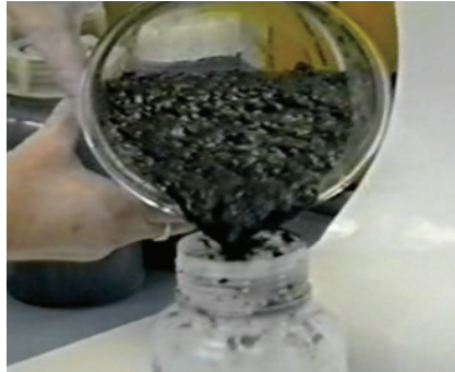
Fig. #5 - Statically Thickened Sludge (~5% TSS)
